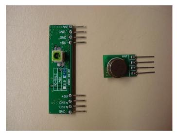
The RF module, as the name suggests, operates at Radio Frequency. The corresponding frequency range varies between 30 kHz & 300 GHz. In this RF system, the digital data is represented as variations in the amplitude of carrier wave. This kind of modulation is known as Amplitude Shift Keying (ASK).
