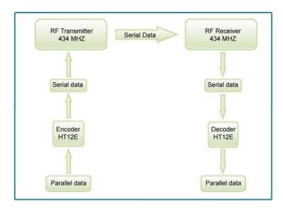
Encoder IC (HT12E) receives parallel data in the form of address bits and control bits. The control signals from remote switches along with 8 address bits constitute a set of 12 parallel signals. The encoder HT12E encodes these parallel signals into serial bits. Transmission is enabled by providing ground to pin14 which is active low. The control signals are given at pins 10-13 of HT12E. The serial data is fed to the RF transmitter through pin17 of HT12E.
