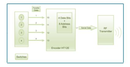
Transmitter, upon receiving serial data from encoder IC (HT12E), transmits it wirelessly to the RF receiver. The receiver, upon receiving these signals, sends them to the decoder IC (HT12D) through pin2. The serial data is received at the data pin (DIN, pin14) of HT12D. The decoder then retrieves the original parallel format from the received serial data.
