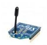
• operate within the ISM 2.4 GHz frequency band
