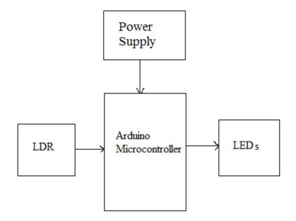
The project uses LEDs as streetlights. An LDR is used to sense the atmospheric light conditions. When it is dark, the LDR has high resistance and a high voltage is dropped across the microcontroller ADC pins. This voltage is converted to its digital value and it is used to drive the LEDs ON. When there is sufficient lighting, the LDR has low resistance and a low voltage is dropped across ADC pins. This keeps the LEDs in OFF condition.
