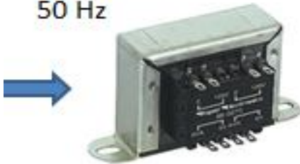
12V step down transformer
