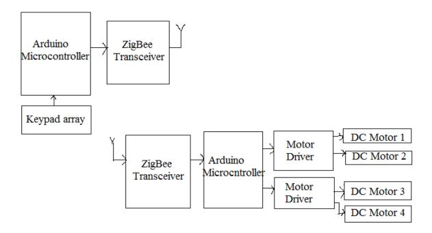
A keypad array of pushbuttons is used to send the control signals to control the robot movements using ZigBee module. At the receiver side the Arduino microcontroller drives the motors used for robotic forward and backward motion and for the robotic arm movement.
