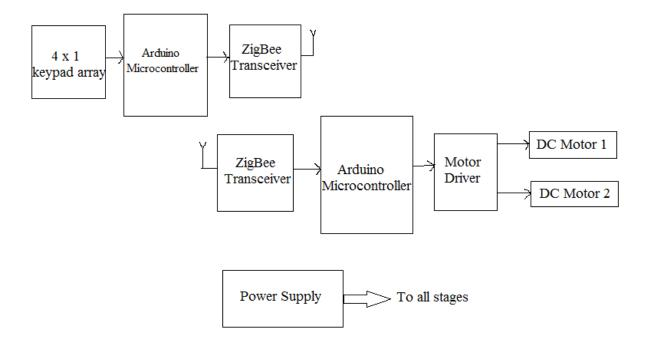
At the transmitter side, there is a  $4 \times 1$  keypad array which is connected to a ZigBee transceiver. At the receiver side, there is a ZigBee transceiver, Arduino microcontroller, Motor Driver and two DC motors. On pressing the pushbuttons of keypad array, the two dc motors can be made to rotate in different directions.
